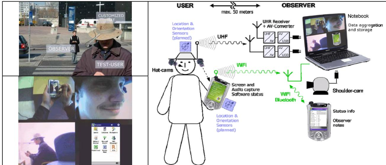
**FIGURE 1:** LiLiPUT System in the field (top left), captured video signals (bottom left) and system architecture (right). Features planned for the future are coded in blue.
