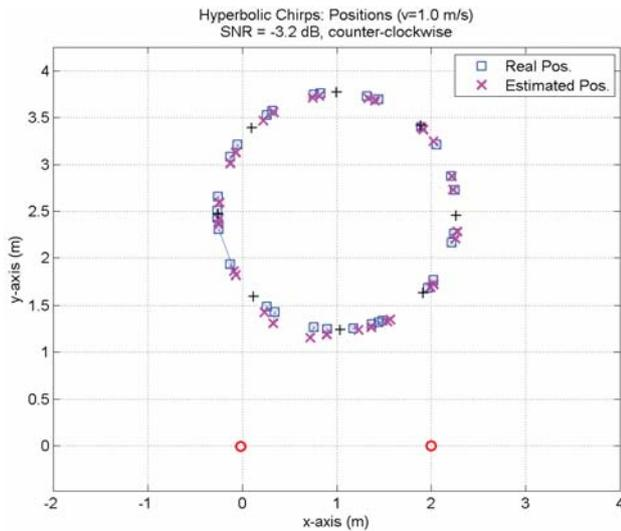
Fig. 6. Position estimates of the system based on hyperbolic (HFM) chirps at the tag moving counter-clockwise at a speed of 1.0 m/s and an SNR of -3.2 dB. The red circles denote the loudspeakers.
