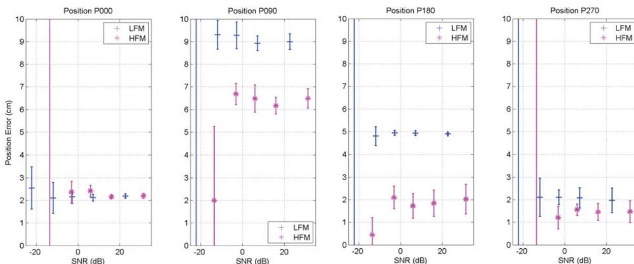
Fig. 3. Position errors vs. SNR of LFM (+) and HFM (\*) signals at positions P000 to P270. The results are apparently biased due to inaccuracies in the ground truth data. However, the precision lies below 7 mm down to an SNR of -3.2 dB.
