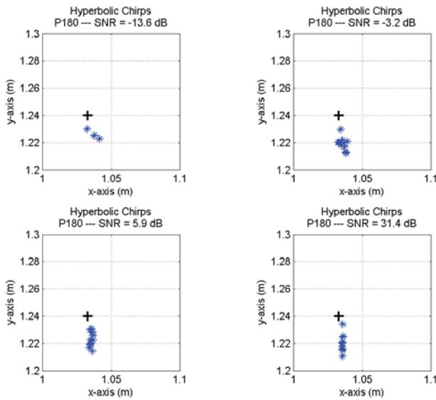
Fig. 4. Position estimates at position P180 at four SNR levels resulting from stationary measurements using HFM chirps. The results are biased but exhibit high precision. Similar results were obtained using the LFM signals.
