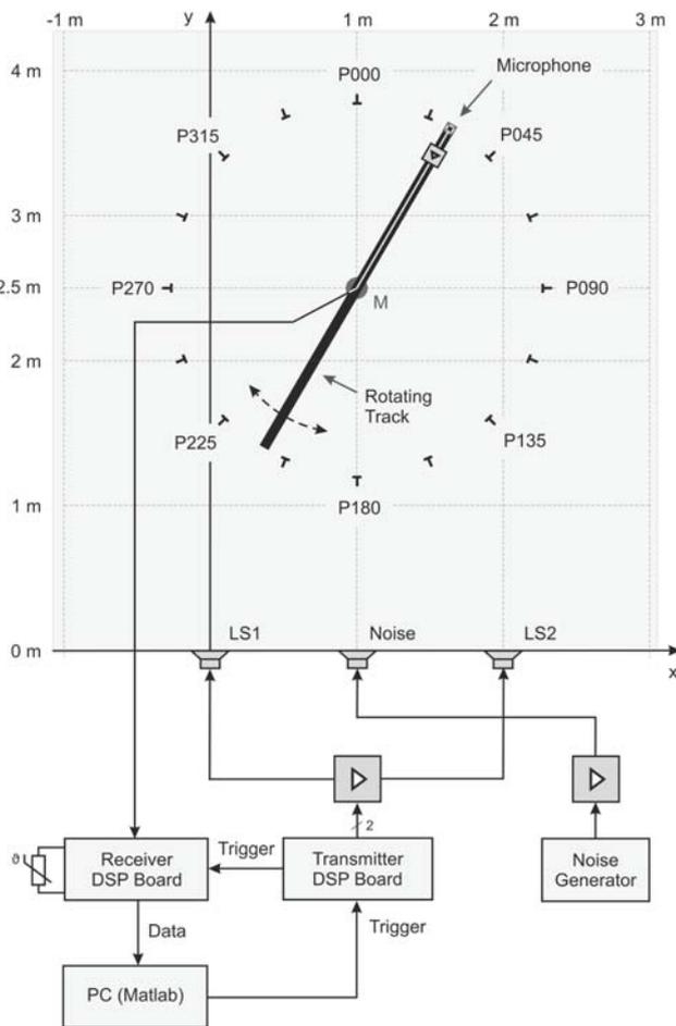
Fig. 2. Measurement setup applying a rotating beam. Upon a trigger from the measurement PC, the transmitter DSP board started to play out the measurement signals and simultaneously triggered the recording at the receiver DSP board. Moreover, the PC controlled the rotation speed of the beam.
