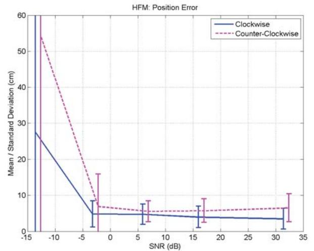
Fig. 7. Position estimation errors vs. SNR using HFM signals at a velocity of 1 m/s for clockwise direction (solid) and counter-clockwise direction (dashed).
