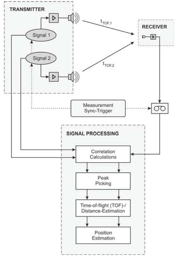
Fig. 1. Acoustic positioning principle. Two measurement signals are transmitted via loudspeakers, while, synchronously, the microphone signal at the receiver is recorded. From the correlation signals of the recorded signal with the original signals, the distances between the loudspeakers and the microphone can be calculated. Finally, the position of the microphone is estimated using bilateration.
