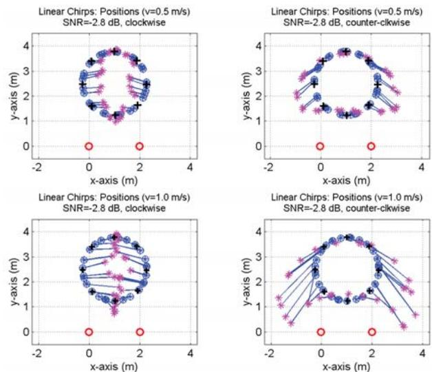
Fig. 5. Position estimates using one LFM up-chirp signal per loudspeaker at an SNR of -2.8 dB. The top plots give the results for a velocity of 0.5 m/s in clockwise and counter-clockwise direction, while the bottom plots show the estimates for a velocity of 1.0 m/s. These figures very well illustrate the impact of the Doppler-shift on the position estimates. The red circles denote the loudspeakers.
